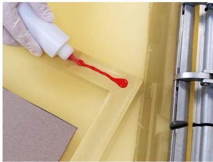
DYNABOND Two-Part Frame Adhesive used after stretching
