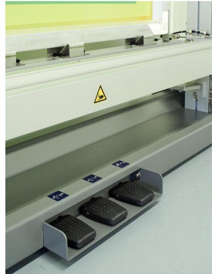
Foot Pedal Controls for Screen Tie-Bar and Stretchers
