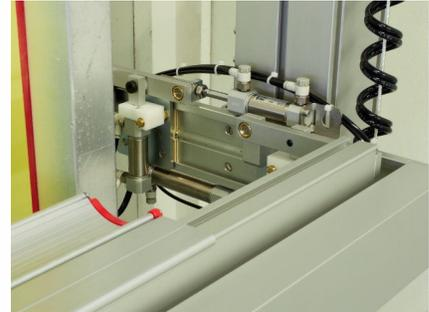
Pneumatically Controlled Coating Carriage
