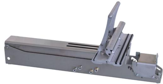
The G-STRETCH 202 PLUS stretching process includes automatic pre-stressing of the screen frame, while the mesh itself is stretched off-contact from the frame. After reaching the preprogrammed tension value, the mesh can be lowered onto the frame with a preset amount of pressure.
