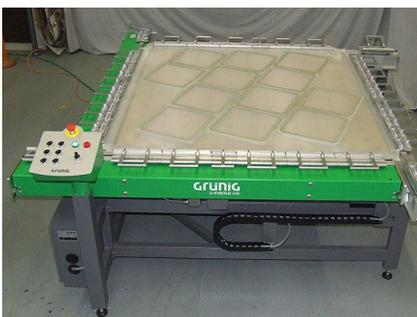
Stretching Multiple Screens Simultaneously
