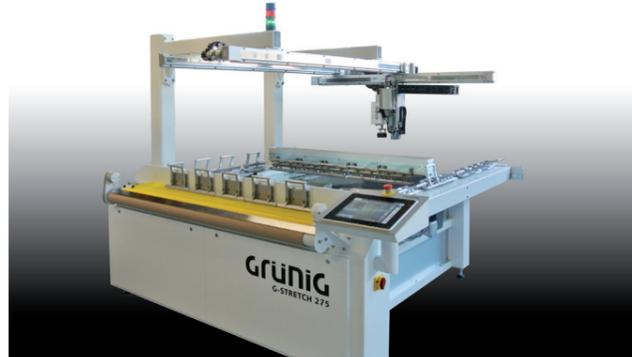
G-STRETCH 275 UV BOND LED: Efficient screen manufacturing in top quality
