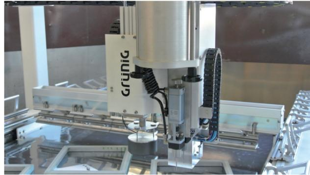
Multi-functional gluing head: measuring, gluing and curing
