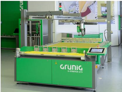
Complete G-STRETCH 275 UV Bond LED Stretching and Gluing System
