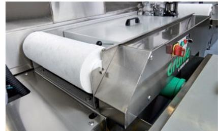
Closed-Circuit Tank with Inclined Filter
