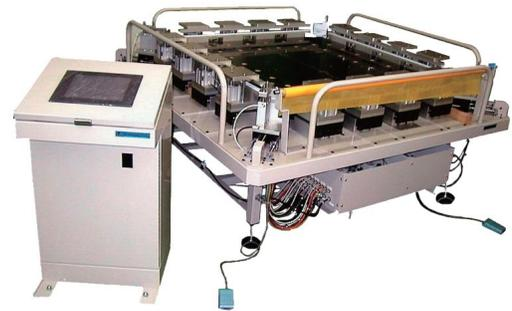
The real ground breaking feature of the Precision Stretcher is its diagonal stretching. Adding tension in the corners is counter to traditional stretching methods, as most stretching equipment adds slack in the corners to avoid tearing the mesh during stretching. However, this conventional approach creates distortion in the corners of the mesh. The Precision Stretcher's novel approach allows for uniform tensioning even in the corners, every time.
