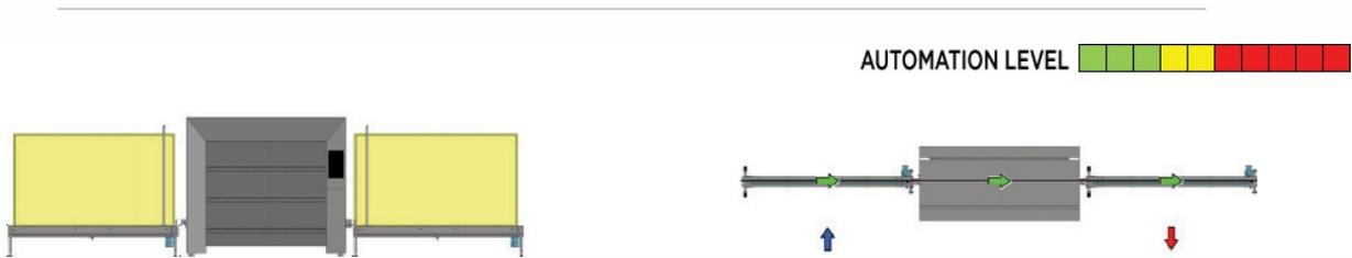
**STM-TEX BASIC-one** is a partially automated configuration that allows for one screen to be exposed while another is loaded. This system includes the following modules:
